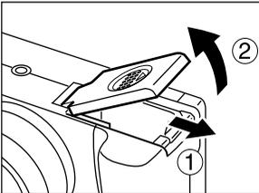
Turn off the power and slide the battery cover in the direction of the arrows (p. 19).
