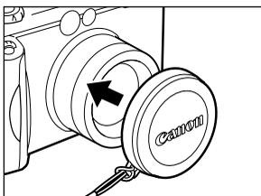
Fit the lens cap over the lens casing so that it covers the entire lens. Always replace the lens cap after use.
