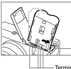
Press the battery lock while inserting the Battery Pack BP-511 and close the battery cover.
