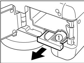
Push point ① with your fingertip while pulling the date battery holder out to remove it.
