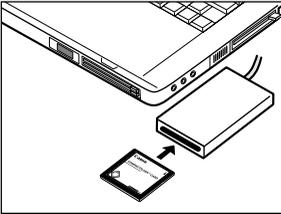
Eject the CF card from the camera, and insert it into a CF card reader connected to the computer.
