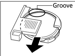
Insert a fingernail into the groove in the date battery and push it out in the direction of the arrow.
