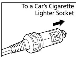
With the engine running, plug the car battery cable into the car's cigarette lighter socket.
