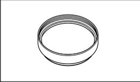
This lens, with a 58 mm-threaded diameter, makes macro shooting easier. With the camera in macro mode, it can shoot subjects as close as 10 cm (3.9 in.) from the lens tip.
