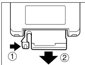
Place your fingertip on ① and press it in the direction of the arrow while placing another fingertip on ② and removing the battery holder.
