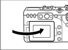
Fold the LCD monitor back against the camera body.
