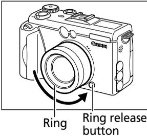
Press the ring release button and remove the ring from around the lens on the camera body.
