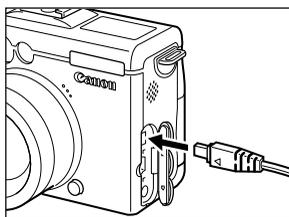
Connect the DC cable to the camera's DC IN terminal.
