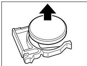
To remove the date battery, pull it in the direction of the arrow.
