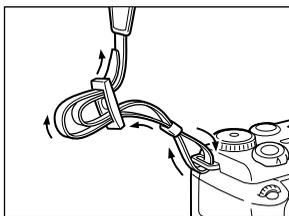
Pass the tip of the strap up through the strap mount on the camera and then through the bottom of the buckle on the strap. Pull the strap tight in the buckle so that it won't slip. Perform the same steps on the other side of the camera.
