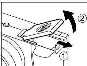
Slide the battery cover in the direction of the arrows.
