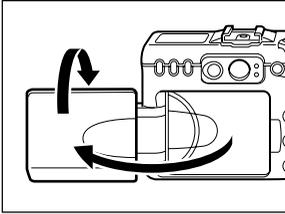
Open the LCD monitor left 180 degrees and tilt it 180 degrees toward the lens.
