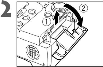
**2** Slide the CF card slot cover in the direction of the arrow and lift it open.
