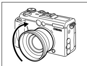
Attach Conversion Lens Adapter so that its • meets the camera's • and turn it in the direction of the arrow.
