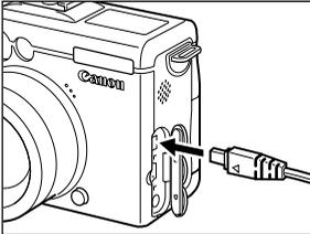
Open the terminal cover and connect the DC plug of the compact power adapter to the camera's DC IN terminal.
