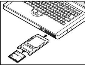
If you are using a PC card reader, first insert the CF card into a PC card adapter (optional), and then insert the PC card adapter into the computer's PC card reader.
