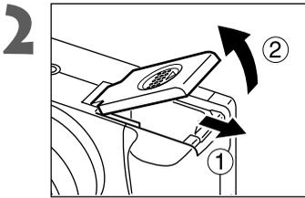
Slide the battery cover in the direction of the arrows.
