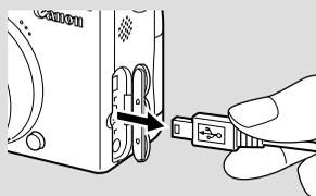
To disconnect the cable from the camera:
