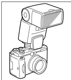
Attach the flash to the camera's hot shoe.
