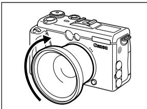
Screw on the lens in the direction of the arrows.
