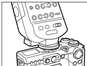
Attach the controller to the camera's hot shoe.
