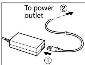
Attach the power cord to the compact power adapter and plug it into power outlet.
