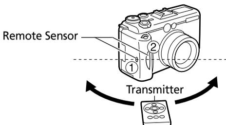
When the Macro Ring Lite MR-14EX or the Macro Twin Lite MT-24EX is mounted on the camera, it will block the front remote sensor (②). In this case, aim the wireless controller toward the side remote sensor (①).
