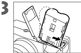
Press the battery lock while inserting the battery pack all the way in until the lock clicks.
