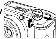
**2** Remove the AA-size batteries, then pull out the battery holder by hooking your fingertip under the bottom of the battery holder edge.
