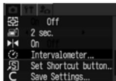
**2** Select an interval time using the ◀ or ▶ arrow.
