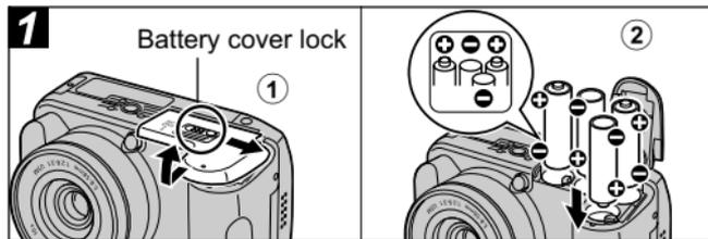
**① Be sure that the camera power is off (p. 19). Slide the battery cover lock in the direction of the arrow and open the cover.**
