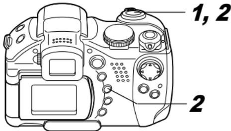
**1 Focus the AF frame or the spot metering frame on the subject on which you wish to lock the exposure setting and press the shutter button halfway.**
