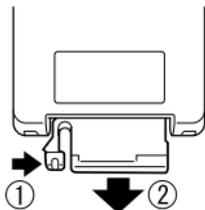
**2** Place the date battery in the battery holder with the negative terminal (-) facing up. Then replace the battery holder into the wireless controller.
