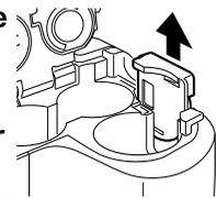
**3** Remove the old date battery and place a new date battery into the date battery holder with the positive terminal (+) facing upward.
