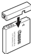
You may be able to check the charge state depending upon how the terminal cover is attached (Fig. C, D).
