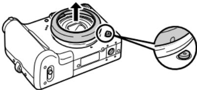
**4 Detach the front section of the conversion lens adapter (p. 112).**
