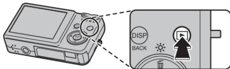
When the camera is off, press
