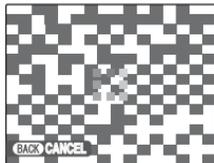
Press DISP/BACK to cancel erasing of all the frames (files). Some unprotected frames (files) will be left unerased.
