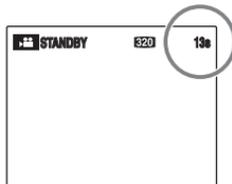
The available recording time appears on the LCD monitor.
