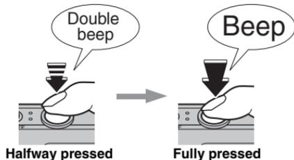
Pressing the shutter button down halfway that focuses on the subject. Without releasing the shutter button, press the button all the way down (fully pressed) to start the self-timer.
