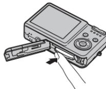
Push the Memory Card into the slot and then slowly remove your finger. The lock is released and the Memory Card is pushed out.
