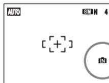
FinePix J10 / FinePix J12 has internal memory that can store images without Memory Card. **IN** appears on the LCD monitor when internal memory is active.
