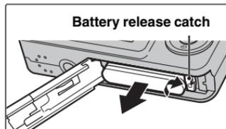
Open the battery cover, and unlock the battery release catch with your finger.
