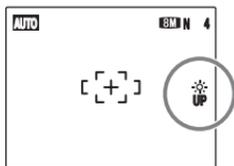
☀ UP blinks on the LCD monitor when the function is on.
