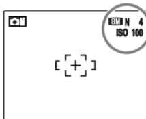
The selected sensitivity setting appears on the LCD monitor when the sensitivity setting is set to another setting excluding [AUTO].
