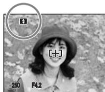
When pressing the shutter button down halfway, **F** appears on the LCD monitor before the flash fires.
