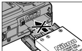
The orange battery latch is pushed aside as the battery is inserted. The latch will close when the battery is fully inserted.
