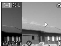
Take first picture. **AE-L** icon is displayed, and **White balance** and **Exposure compensation** are locked. About one third of picture is shown superimposed on view through lens (if pan direction is left to right, picture will appear on left side of monitor).
