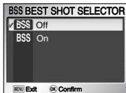
When the “Best Shot Selector” (BSS) is on, the camera takes a maximum of ten pictures as long as the Shutter-release Button is held down. These images are then compared and the sharpest picture (the picture with highest level of detail) is saved to the memory or memory card. BSS is recommended for situations in which inadvertent camera movement can produce blurred pictures, for example when:
