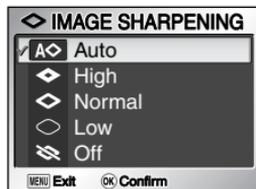
The camera automatically processes pictures to emphasize the borders between light and dark areas of the picture, making edges seem sharper.
