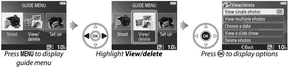
Highlight **View/delete** in the top level of the guide menu and press **OK** to display the following options:
