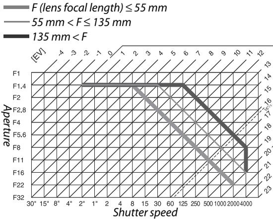
The maximum and minimum values for EV vary with ISO sensitivity; the above graph assumes an ISO sensitivity of ISO 100 equivalent. When matrix metering is used, values over  $16^{1/3}$  EV are reduced to  $16^{1/3}$  EV.
