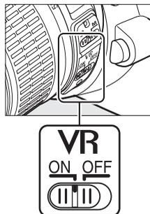
Vibration reduction can be turned off by sliding the VR switch to **OFF**. Turn vibration reduction off when the camera is securely mounted on a tripod, but leave it on if the tripod head is not secured or when using a monopod.
