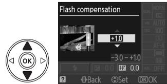
Normal flash output can be restored by setting flash compensation to  $\pm 0$ . Flash compensation is not reset when the camera is turned off.
