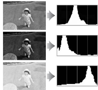
Increasing exposure compensation shifts the distribution of tones to the right, while decreasing exposure compensation shifts the distribution to the left. Histograms can provide a rough idea of overall exposure when bright ambient lighting makes it difficult to see photographs in the monitor.
