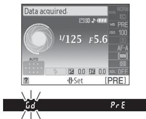
If lighting is too dark or too bright, the camera may be unable to measure white balance. A message will appear in the information display and a flashing **no ūd** will appear in the viewfinder for about eight seconds. Return to Step 4 and measure white balance again.
