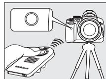
If no operations are performed for about five minutes after selecting delayed remote or quick-response remote modes, the camera will automatically return to single frame or continuous mode, cancelling remote control mode.
