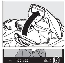
To save battery power when the flash is not in use, return it to its closed position by pressing it gently downward till the latch clicks into place.
