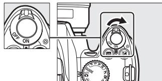
Rotate the power switch as shown to turn the camera off.
