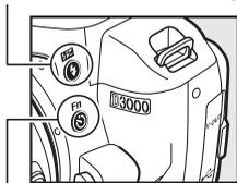
**Fn (C) button:** release mode, image quality and size, ISO sensitivity, white balance, Active D-Lighting, or framing grid display
