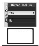
**3** Press the shutter-release button all the way down. The mirror will be raised and the shutter curtain will open, revealing the low-pass filter, and the row of dashes in the control panel will blink.
