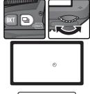
3 Frame the photograph and focus. If autofocus is in effect, be sure not to block the lens when activating the self-timer. In single-servo autofocus (▶ 139), photographs can only be taken if the in-focus (●) indicator appears in the viewfinder
