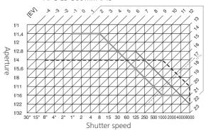
The maximum and minimum values for EV vary with sensitivity (ISO equivalency); the above graph assumes a sensitivity of ISO 200 equivalent. When matrix metering is used, values over 171/3 EV are reduced to 171/3 EV.
