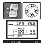
The focus selector lock can be set to  $\mathbf{L}$  (lock) following selection to prevent the selected focus area from changing when the multi selector is pressed.
