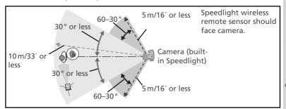
The maximum distance between the optional Speedlights and the camera is about 10 m (33') when the Speedlight is positioned in front of the camera (within 30° on either side of the center line), or about 5 m (16') when the Speedlight is to the side (30–60° to either side of the center line).
