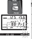
Frame the reference object so that it fills the viewfinder and press the shutter-release button all the way down. The camera will measure a value for white balance and use this value when preset white balance is selected. No photograph will be recorded; white balance can be measured accurately even when the camera is not in focus.
