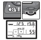
$\mathbf{2}$  Position the subject in the selected focus area and press the shutter-release button halfway (when using center-weighted metering, position the subject in the center focus area). With the shutter-release button pressed halfway and the subject still positioned in the focus area, press the AE-L/AF-L button to lock exposure. Confirm that the in-focus indicator (•) appears in the viewfinder.
