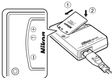
CHARGE lamp starts blinking when battery is inserted ②. Charging is complete when lamp stops blinking ③.
