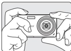
When taking pictures in "tall" orientation, turn the camera so that the built-in flash is above the lens.
