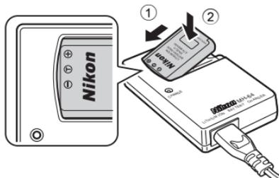
CHARGE lamp starts blinking when battery is inserted ③. Charging is complete when lamp stops blinking ④.
