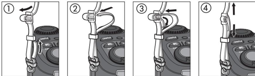
To avoid losing the lens cap, use the cord provided to attach it to the camera strap as shown.
