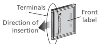
Insert card terminals first with front label facing camera back
