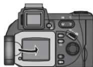
When the monitor is not in use, you can fold it onto the camera body as shown to protect it from dust or fingerprints.
