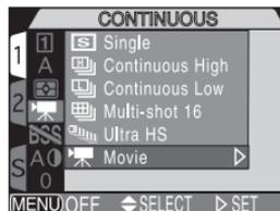
**2** Press the shutter-release button all the way down to begin recording. If the monitor is rotated to point in the same direction as the lens, the image in the monitor will be inverted. The exposure count display will show the length of the movie that can be recorded.
