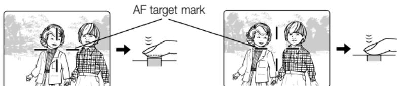
Position your main subject inside the AF target marks, and press the shutter button down halfway.
