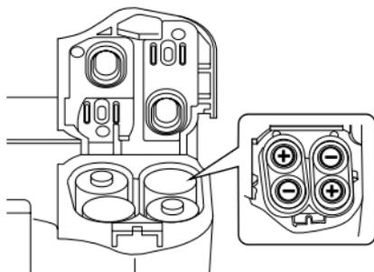
When using AA-size batteries
