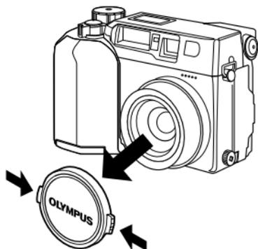
To switch the camera on, remove the lens cap and set the Mode dial to any setting other than OFF.
