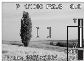
The cursor moves up and down the zoom indicator according to the zoom magnification. The cursor turns orange when inside the digital zoom area.
