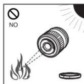
Do not leave the lens without the cap. If solar light is converged through the lens, a fire may result.
