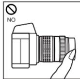
Do not hold the camera by the section of the lens extruded by the focusing operation.
