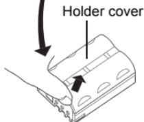
**3** Insert the batteries into the battery holder in the direction shown in the illustration.
