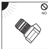
Do not point the camera lens at the sun. Sunlight will converge in the lens and focus inside the camera, possibly causing a malfunction or fire.
