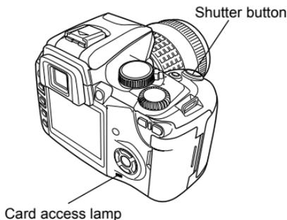
**2 Press the shutter button halfway until the AF confirmation mark lights.**
