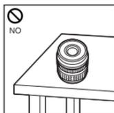
Do not put the lens with its contacts facing down.
