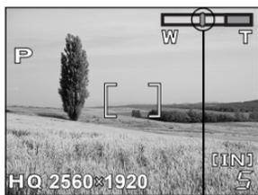
The cursor moves left and right on the zoom indicator according to the zoom magnification.
