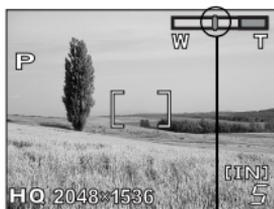
The cursor moves left and right on the zoom indicator according to the zoom magnification.
