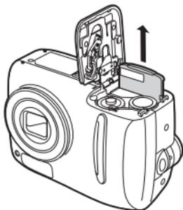
**4 Holding the batteries down with the battery compartment/card cover, close the cover in the direction of ③ and slide it in the direction of ④.**
