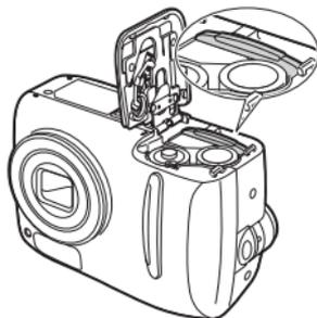
The position of the card inserted correctly
