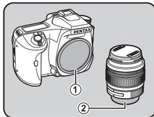
**3 Align the red dots on the camera and the lens, and secure by turning the lens clockwise until it clicks.**
