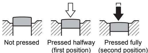
Pressing it down halfway (first position) turns on the viewfinder and LCD panel indicators and the autofocus system operates. Pressing it fully (second position) takes the picture.
