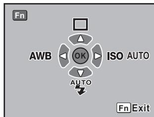
Press the four-way controller (⬆️⬅️⬇️➡️) to set the operation.
