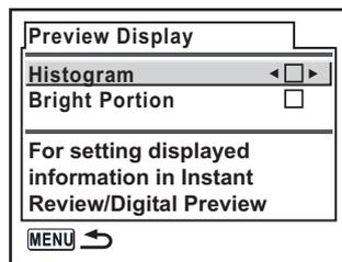
**3** Use the four-way controller (⬅️) to select  (On) or  (Off) for [Histogram].
