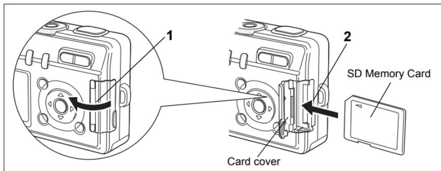
This camera uses an SD Memory Card. Captured images are recorded on the SD Memory Card if a card is inserted (☐ appears on the LCD monitor) or in the built-in memory if no card is inserted (📷 appears on the LCD monitor). Make sure that the camera is turned off before inserting or removing the SD Memory Card.
