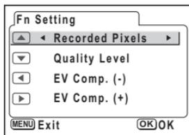
The default settings are as follows: Recorded Pixels on ▲, Quality Level on ▼, EV Compensation (-) on ◀ and EV Compensation (+) on ▶. Select [Off] if you do not want to register a function.
