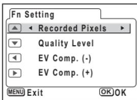
The default settings are as follows: Recorded Pixels on ▲, Quality Level on ▼, EV Compensation (-) on ◀ and EV Compensation (+) on ▶. Select [Off] if you do not want to register a function.
