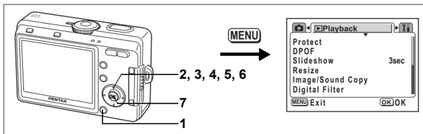
You can copy image and sound files from the built-in memory to the SD Memory Card and vice versa. This function can only be selected when a card has been inserted in the camera.
