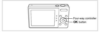
Press the four-way controller (◄) in ♠ mode.
