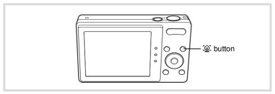
An icon indicating either Face Detection On or Smile Capture appears on the display. (The icon does not appear when the Face Detection function is not activated.)
