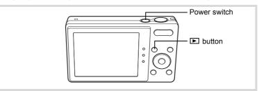
Press the power switch while holding down the button.
