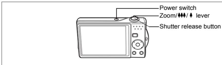
The standard procedure for taking still pictures is described below. The flash discharges automatically depending on the light conditions.
