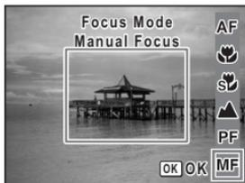
**2 Use the four-way controller (▶) to select MF and press the OK button.**
