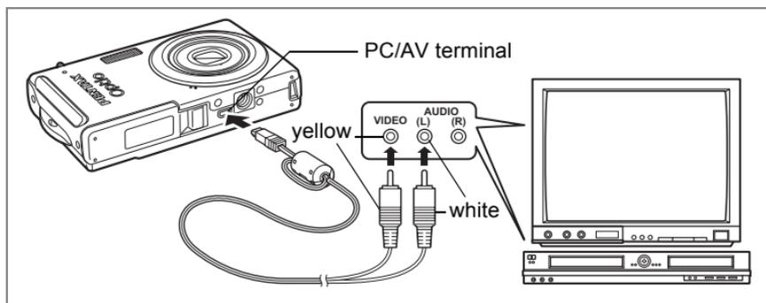
By using the AV cable, you can take pictures and play back captured images on equipment with a video IN jack, such as a TV. Make sure the camera and TV are turned off before connecting the camera to the TV.
