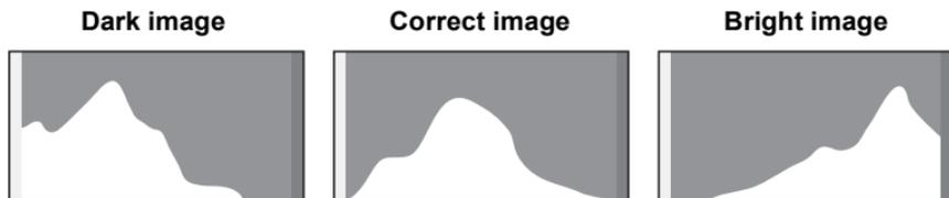
When the image is too dark, the part to the left is cut off (dark portions) and when the image is too bright, the part to the right is cut off (bright portions).
