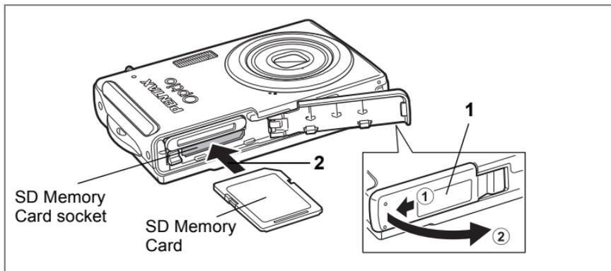
This camera uses either an SD Memory Card or an SDHC Memory Card. (Both cards are referred to as SD Memory Cards hereafter.) Captured images and sound files are saved on the SD Memory Card if a card is inserted in the camera. They are saved in the built-in memory if a card is not inserted. (p.32)
