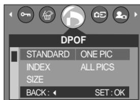
4. Use the UP and DOWN buttons to select [ONE PIC] or [ALL PICS], and then press the OK button.
