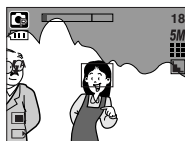
2. Press the SHUTTER button halfway and focus on the subject.
