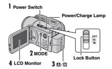
Set the appropriate operation mode according to your preference using the power and MODE switches and > (M/M) button.
