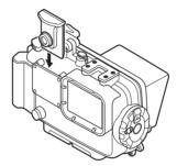
② Put the underwater optical fiber cable plug all the way into the insertion slot of the optical fiber cable adapter until the black axis of the connector is hidden.
