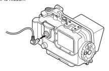
Remove the optical fiber cable adapter when you do not use an underwater optical fiber cable while taking picture.
