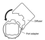
2 Install the strap of the port adapter to the Case body.
