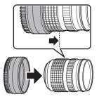
5. Attach the antireflective ring to the lens.
