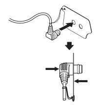
② Put the cap to the optical fiber cable insertion slot when not in use.
