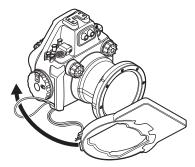
③ Install the diffuser on the Case.
