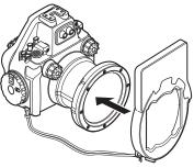
Removing diffuser (with port adapter) from the Case body To remove the diffuser, pull the port adapter from the
