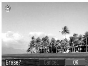
3 Press the ◀ or ▶ arrow on the omni selector to select [OK] and press the Set button.
