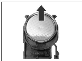
To remove the button battery, pull it in the direction of the arrow.
