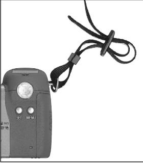
Pass the tip of the strap through the inside slots in the fastener after passing it through the camera eyelet. Take the slack out of the strap above and below the fastener to prevent it from slipping.
