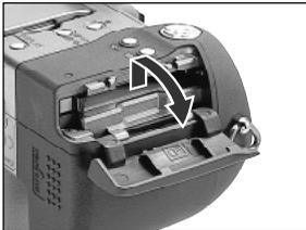
2 Slide the CF card slot cover in the direction of the arrow and lift it to open.
