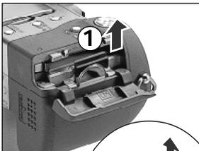
3 Insert a fingernail at ① in the diagram and lift up to remove the button battery holder.
