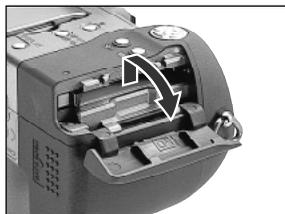
2 Slide the CF card slot cover in the direction of the arrow and lift it open.
