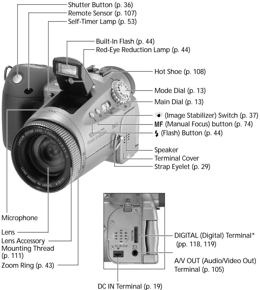
\* To connect the camera to the computer with the USB interface, attach the supplied USB cable to the camera's Digital terminal. To connect to a serial port, the separately sold serial cable (IFC-200PCS for Windows and IFC-200MC for Macintosh) is required.
