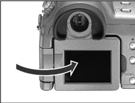
**2** Fold the LCD monitor back against the camera body.
