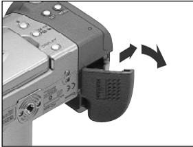
2 Slide the battery cover lock in the direction of the arrow and lift to open it.
