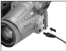
**1** Attach the power cord to the compact power adapter and plug it into an electrical outlet.
