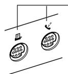
Serial ports (printer, modem) are identified with these symbols.
