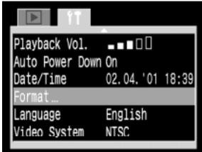
1 In the **[SET UP]** (Set up) menu, select **[Format]** and press the Set button.
