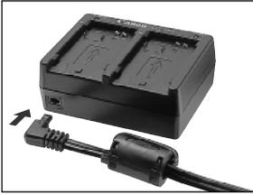
**1** Attach the car battery cable to the charge adapter.
