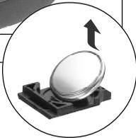
4 Remove the battery from the holder by pulling it in the direction of the arrow.
