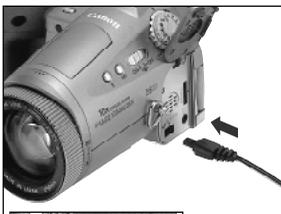
5 Connect the DC plug of the compact power adapter to the camera's DC IN terminal.
