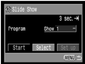
2 Press the or arrow on the omni selector to select [Program]. Press the or arrow to select [Show 1], [Show 2] or [Show 3] and press the Set button.
