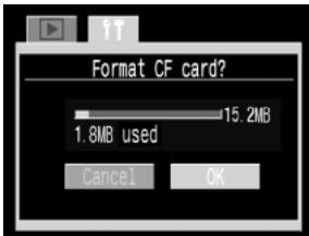
2 Press the **[LEFT]** or **[RIGHT]** arrow on the omni selector to select **[OK]** and press the Set button.
