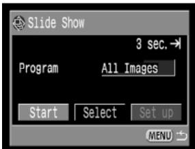
2 Press the [▲] or [▼] arrow on the omni selector to select [Program]. Press the [◀] or [▶] arrow to select between [All Images] or any one of slide [Show 1]-[Show 3].
