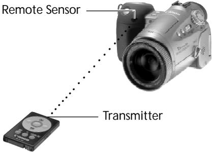
The wireless controller can be used to shoot or replay. Use within approximately 5 m (16.4 ft.) of the remote sensor.
