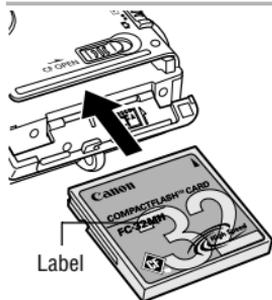
**2** Insert the CF card with its label facing upward until the CF card eject button fully extends.
