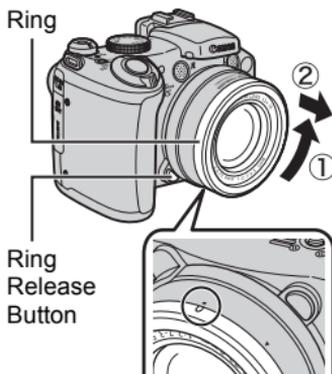
**3** Align the ● mark on the conversion lens adapter with the ● mark on the camera, and turn the adapter in the direction of the arrows until locked (as far as the ▲ mark on the camera).
