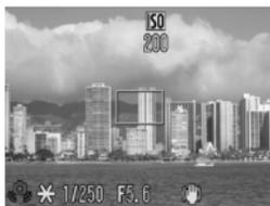
**3 Press the ◀ or ▶ button until the desired shutter speed or aperture value is reached.**
