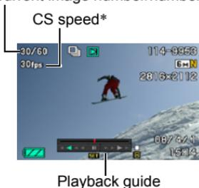
\* The CS speed does not appear on the monitor screen in the high-speed CS mode while "AUTO-N" or "AUTO-H" is selected as the CS speed, or on images shot in the bracketing mode.
