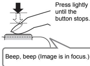
When you half-press the shutter button, the camera automatically adjusts exposure and focuses on the subject it is currently pointed at. Mastering how much pressure is required for a half-press and a full-press of the shutter button is an important technique for good-looking images.
