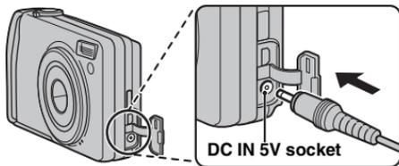
Check that the camera is off. Plug the AC power adapter connector into the DC IN 5V socket and then plug the AC power adapter into the power outlet.
