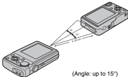
③ Point the camera's infrared port towards the front of the camera's infrared port (→p.13). Transmission distance is about 5 to 20 cm (2 to 7.9 in.) within approx. 15°.
