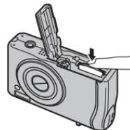
Push the Memory Card into the slot and then slowly remove your finger. The lock is released and the Memory Card is pushed out.
