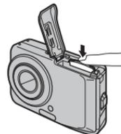
Push the Memory Card into the slot and then slowly remove your finger. The lock is released and the Memory Card is pushed out.
