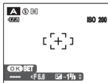
When the brightness of the subject is outside the camera's brightness metering range, [----] appears as the shutter speed. When this occurs, press the shutter button down halfway to measure the light level again.
