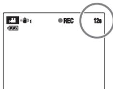
Press the shutter button down fully to start recording. During recording, [●REC] and a counter that shows the remaining time appear on the LCD monitor.
