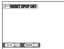
When the data includes a frame (file) with DPOF settings that were specified on another camera, [
