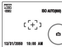
FinePix F50fd has internal memory that can store images without Memory Card. **iN** appears on the LCD monitor when internal memory is active.
