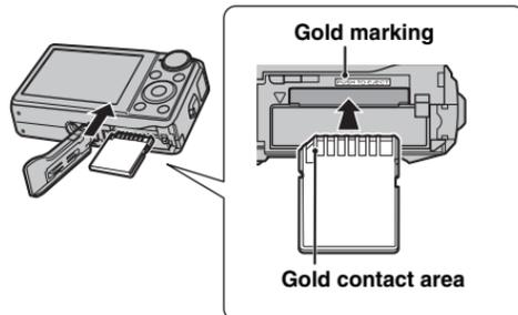
Align the gold marking with the gold contact area, then insert an SD Memory Card completely.
