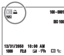
The camera icon with a face appears on the LCD monitor during playback when the image has specified DPOF settings.
