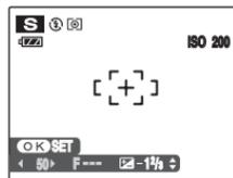
When the brightness of the subject is outside the camera's brightness metering range, [F---] appears as the aperture setting. When this occurs, press the shutter button down halfway to measure the light level again.
