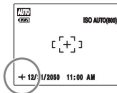
In the time difference setting, when you change to the Photography mode, + and the date is displayed for 3 seconds, the date display turns yellow.
