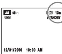
The available recording time appears on the LCD monitor.
