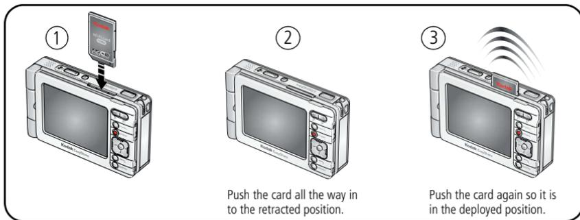
When possible, keep the Wi-Fi card in the retracted (2) position for safe-keeping and to conserve battery life. To connect to an available Wi-Fi wireless network, push the card in so that it springs back up to the deployed (3) position (see page 44).
