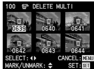
8. Mark each picture to be deleted individually by pressing up on the direction pad.
