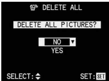
7. Press up or down on the direction pad to select **NO** to retain a picture or **YES** to delete.
