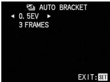
4. Select the desired exposure graduation between the individual pictures by pressing left or right respectively on the direction pad to increase or decrease the graduation.
