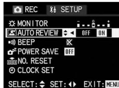
5. Select **OFF** or **ON** by pressing left or right on the direction pad.
