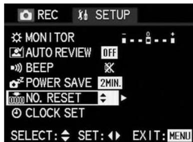
5. Open the corresponding sub-menu by pressing right on the direction pad.
