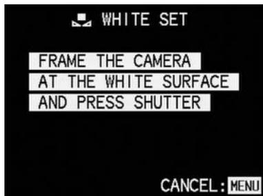
8. Aim the camera at an object which you know is white or neutral grey. It should fill the frame in the monitor.
