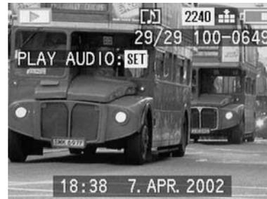
3. To play back the recording, press the **VIEW/SET** button (1.31). During playback, the line **PLAY AUDIO SET** in the monitor disappears, and The red LED (1.20) is lit constantly.
