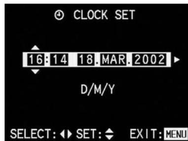
5. Press right on the direction pad again to select the first data item to be set. This data item is identified by arrows pointing upwards and downwards.
