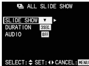
7. Press up or down on the direction pad to select **DURATION 3SEC**.
