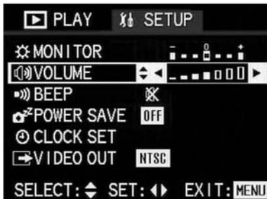
5. Select the desired volume by pressing left or right on the direction pad. 6 levels are available, with the height of the bar representing the volume. The setting is shown by the bar being marked in yellow.
