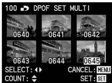
7. Select each picture to be marked individually by pressing left and/or right on the direction pad. The number of the active picture is always shown in yellow.
