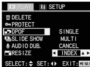
6. Open the associated sub-menu by pressing right on the direction pad.
