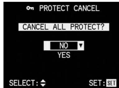
7. Press up or down on the direction pad to select **NO** to retain or **YES** (marked with upwards arrow and in yellow, if activated) to delete all protection settings.
