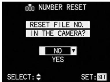
6. Select **NO** to retain the existing folder number or **YES** (marked with the upwards arrow and in yellow if activated) for a new number by pressing up or down on the direction pad.
