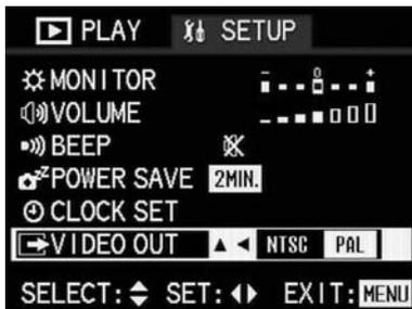
5. Select **NTSC** or **PAL** by pressing right or left on the direction pad. The active setting is marked in yellow.
