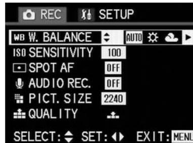
press right on the direction pad to access the appropriate basic setting menu (**SETUP**).
