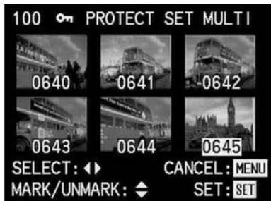
7. Select each picture to be protected individually by pressing left and/or right on the direction pad.
