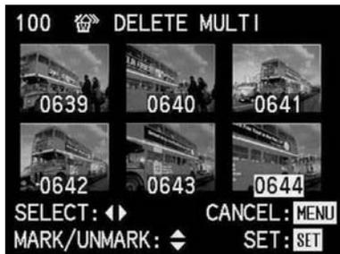
7. Select each picture to be deleted individually by pressing left and/or right on the direction pad. The number of the active picture is always shown in yellow.
