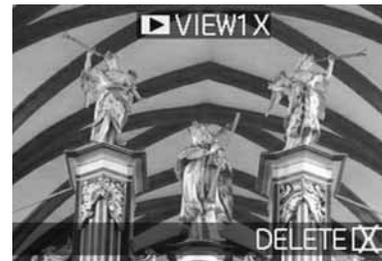
At any time, you can return to the original viewfinder/monitor screen, and thus to immediate readiness to take a picture by pressing the shutter release button (1.13), or by pressing the direction pad down again.
