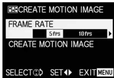
5. Select the desired picture frequency for playback (**FRAME RATE**) and then save the series of pictures (**CREATE MOTION IMAGE** again) according to the menu instructions.
