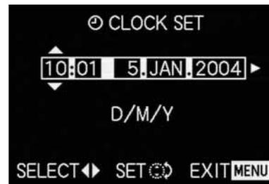
3. Use the direction pad or the central adjustment dial to set the desired numeric value. The other numeric values and the month are selected with the direction pad and then set in basically the same way.
