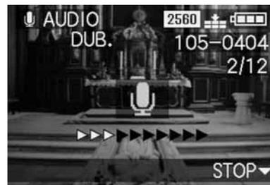
**Note:** If there is insufficient memory capacity on the card to add a sound recording, the picture in the background disappears for a short time, the monitor screen turns blue and **NOT ENOUGH MEMORY ON CARD** appears.
