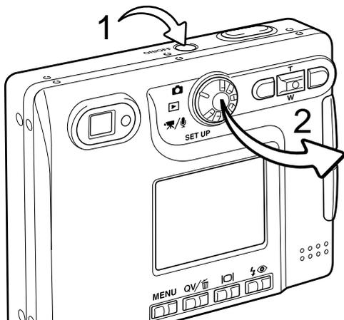
Turn the camera on by pressing the main switch near the shutter-release button (1).
