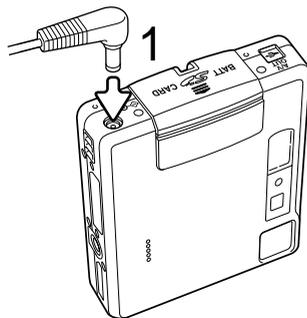
The AC adapter AC-4 or AC-5 allows the camera to be powered from a household outlet. The AC adapter is recommended when the camera is interfaced with a computer or during periods of heavy use. AC adapter model AC-4 is for use in North America, Japan, and Taiwan, and AC-5 is for use in all other areas. The battery cannot be charged using the AC adapter.
