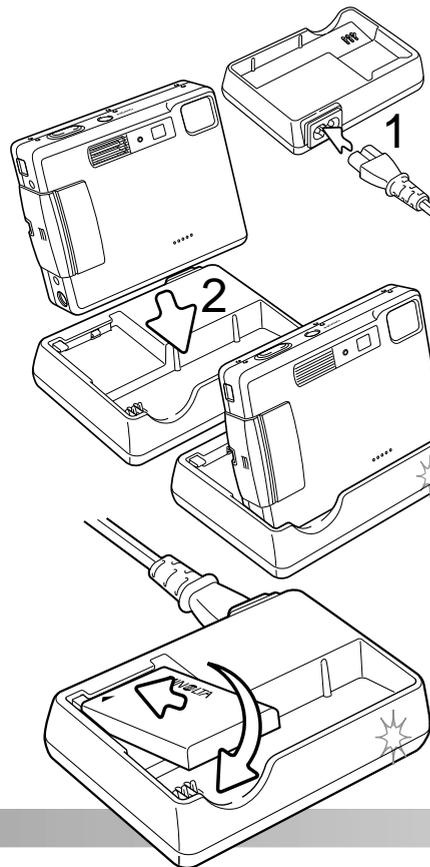
Plug the power cord into the back of the charger unit (1). Plug the other end of the cord into a live household outlet. The included AC cord is designed for the current of the sales region. Only use the cord in the region it was purchased. For more on the AC cable, see page 104.
