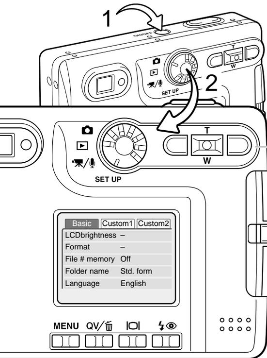
Turn the camera on by pressing the main switch near the shutter-release button (1).
