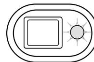
The indicator lamp next to the viewfinder can be used to diagnose camera operations. The lamp colors change between green, red, and orange, and the lamp can glow steadily or blink at two rates.
