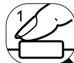
Press the shutter-release button partway down (1) to lock the focus and exposure.
