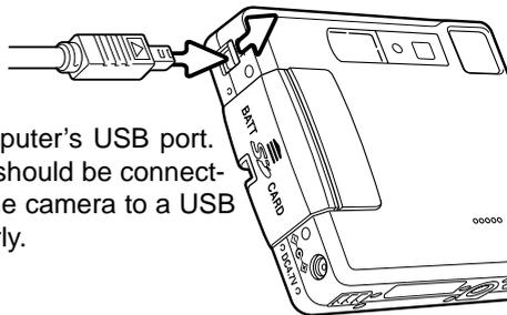
4. Attach the other end of the USB cable to the computer's USB port. Make sure the plug is firmly attached. The camera should be connected directly to the computer's USB port. Attaching the camera to a USB hub may prevent the camera from operating properly.
