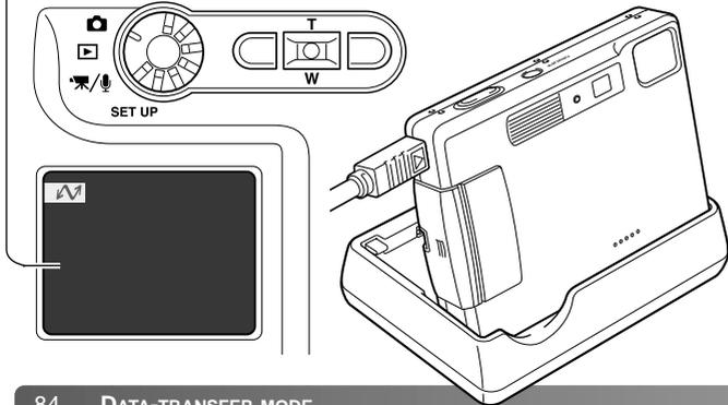
The charger can be used as a camera stand. When the camera is on, the charger does not charge or supply power to the camera.
