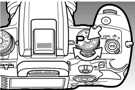
While pressing the dial release, turn the exposure dial to the program (P) position. The camera controls the exposure system.
