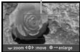
The magnification area (3) shows the portion of the image enlarged. The controller's four-way keys scrolls the magnification area. The rear control dial changes the size of the area.
