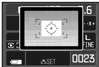
On the register-selection screen use the control dials or left/right keys of the controller to select the custom white-balance register in which to store the setting; any previous setting is replaced. Press the central button of the controller to complete the operation.
