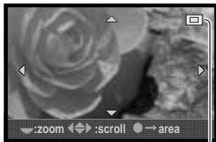
The controller's four-way keys scrolls the magnified area. The locator (2) indicates the portion of the image displayed. The rear control dial changes the magnification.
