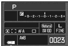
This camera is equipped with an automatic battery-condition indicator. When the camera is on, the indicator appears on the monitor. The indicator changes from white to red when battery power is low. If the monitor is blank, the battery may be exhausted.
