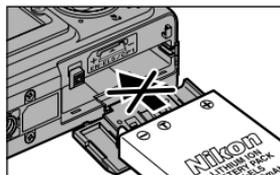
The orange battery latch is pushed aside as the battery is inserted. The latch will close when the battery is fully inserted.
