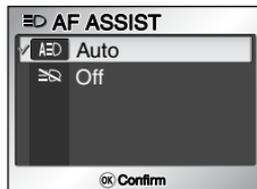
Your camera is equipped with an AF-assist Illuminator. If lighting is poor, the built-in AF-assist Illuminator will light when the shutter-release button is pressed halfway, allowing the camera to focus even when the subject is poorly lit. Select **Auto** (default setting) or **Off** and press **OK**.
