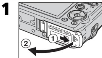
Open battery chamber/memory card slot cover. Slide the cover until it stops (1) and open it (2).
