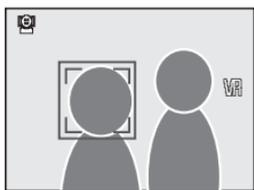
Press shutter-release button halfway to set focus and exposure.
