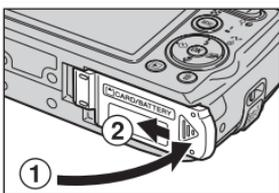
Close battery chamber/memory card slot cover. Close the cover (①) and slide it until it latches (②).
