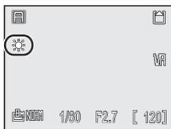
If white balance is set to an option other than **Auto**, rotate mode dial to **P** or **A**.
