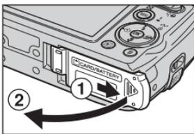
Confirm that camera is off and open battery chamber/memory card slot cover. Slide the cover until it stops (①) and open it (②).
