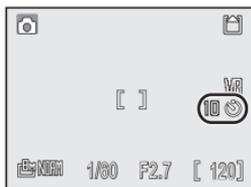
Press shutter-release button the rest of the way down to start timer.
