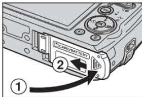
Close battery chamber/memory card slot cover. Close the cover (①) and slide it until it latches (②).
