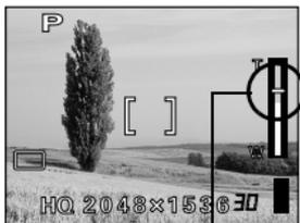
The cursor moves up and down on the zoom indicator according to the zoom magnification.
