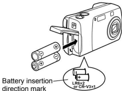
There is a mark showing the correct way to insert the AA batteries on the bottom of the camera.
