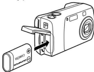
When using a CR-V3 lithium battery pack, insert it in the direction as shown in the illustration.
