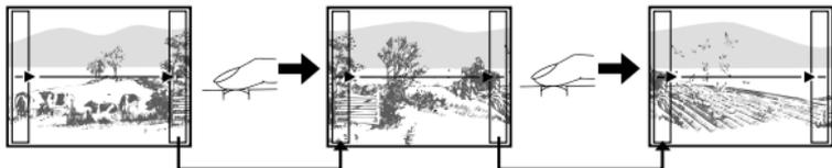
When shooting, make sure that the edges (right/left/top/bottom) of the images overlap, so that the CAMEDIA Master software can correctly connect the pictures.
