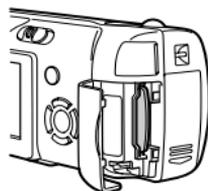
The position of the card inserted correctly
