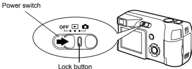
**Power off:** Slide the power switch to OFF.
