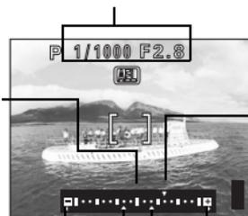
Indicates how much the present exposure you are metering differs from the average exposure value. The present exposure can be fixed by pressing the shutter button halfway. (The present exposure is not added to the average value unless you press **AEL** /
