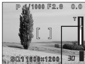
The cursor moves up and down on the zoom indicator according to the zoom magnification. The cursor turns orange when inside the digital zoom field.
