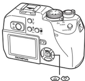
If the aperture value is displayed in red, the aperture setting is unsuitable for the conditions. Take the following steps. (When the aperture value is displayed in green, the setting will provide optimum exposure.)
