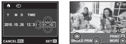
Operation guides displayed at the bottom of the screen indicate that the **MENU** button, **OK** button, or zoom buttons can be used.
