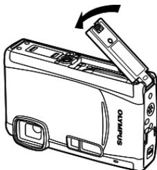
⚠ Please ensure that foreign material such as dirt and sand, etc, does not stick to the gasket of battery/card compartment cover and that there are no cracks and scratches.
