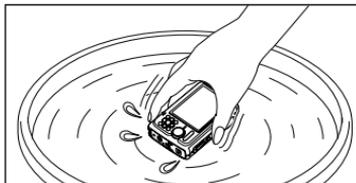
Follow the Steps ① to ④, then check if the lens cover moves smoothly. If the lens cover does not move smoothly, rinse the lens face by placing it directly under a strong stream of tap water and pressing the **ON/OFF** button repeatedly.
