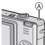
**1 Press and hold the optical image stabilizer button (A) until [STABILIZER] appears and then select the stabilizer function mode.**
