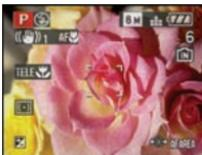
If you zoom to a magnification of 12× to 18× (close to Tele), you can take a picture of an object that is only 1 m (3.28 feet) from the lens. (The tele-macro icon [
