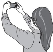
Press [HIGH ANGLE] **(A)** for 1 second to display the High angle mode icon **(B)**.
