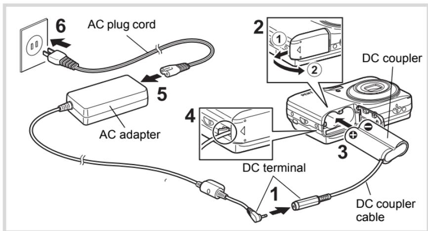
**1** Connect the DC terminal of the AC adapter to the DC input terminal of the DC coupler.
