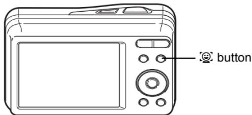
An icon indicating Face Detection On or Smile Capture appears when switched to either face detection function. (The icon does not appear when the Face Detection function is not activated.)
