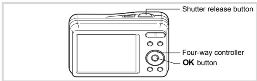
**1** Press the four-way controller () in mode.
