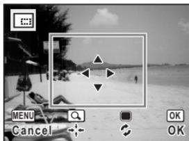
The following operations move the green frame and set the area for cropping on the screen.
