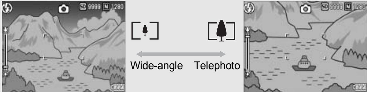
**1** With the camera ready to shoot, press the [▲] (Wide-angle) button or the [▼] (Telephoto) button.
