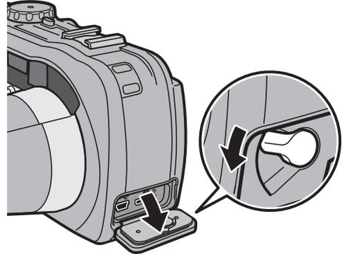
**3** Connect your camera to a printer using the USB cable provided.
