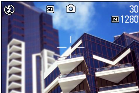
If the camera cannot automatically focus, the crosshairs in the center of the LCD monitor turn red and the auto-focus lamp in the lower left of the viewfinder blinks in green.
