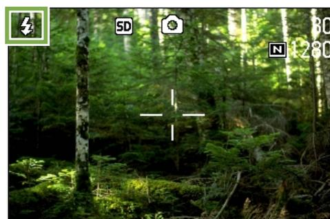
The flash starts recharging. While the flash is charging, the LCD Monitor goes off and the flash lamp blinks. Once charging is complete, the lamp remains lit and it is possible to shoot.
