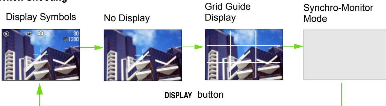
AEIn the Synchro-Monitor Mode except with the following operations, the LCD Monitor is turned off (No Display). This is a useful mode to reduce power consumption.
